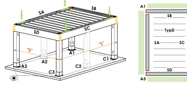
SA, SC – Perimeter frame – Length SB, SC – Perimeter frame – Width A1, A3, C1, C3 – Corner poles A2, C2 – Additional poles "S" – Maximum pergola width "L" – Maximum pergola length
