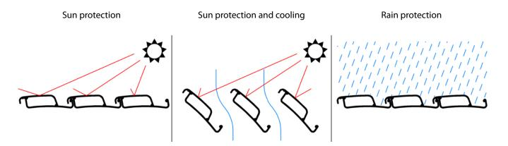
The bioclimatic pergola is a shading element intended as sun protection. Slat tilting allows ventilating the space under the roof while retaining the shading function. The pergola also serves as rain protection. However, water-resistance is limited due to the product design. Detailed information can be found in the section Basic specification – Water resistance.
