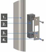
1. U-section with slot 2. Lock counterpart – plastic 3. Lock counterpart – stainless 4. Screw 3.9 × 32
