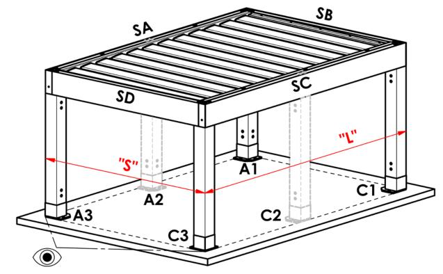
SA, SC – Perimeter frame – Length SB, SC – Perimeter frame – Width A1, A3, C1, C3 – Corner poles A2, C2 – Additional pole
