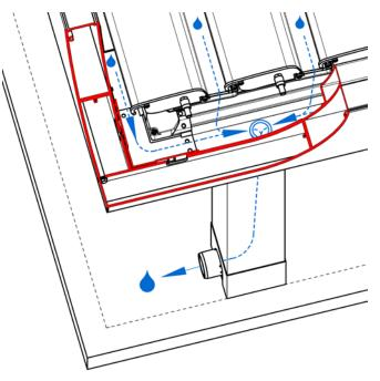
Water flow direction to the pole with a drain located outside the pergola corner Water flow direction to the pole with a drain located in the pergola corner
