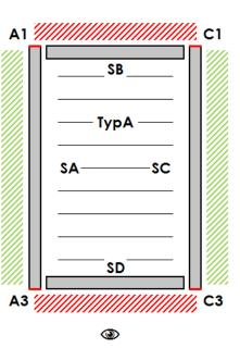
SA, SC – Perimeter frame – Length SB, SC – Perimeter frame – Width A1, A3, C1, C3 – Corner poles A2, C2 – Additional poles
