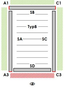
SA, SC – Perimeter frame – Length SB, SC – Perimeter frame – Width A1, A3, C1, C3 – Corner poles A2, C2 – Additional poles "S" – Maximum pergola width "L" – Maximum pergola length
